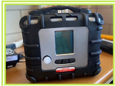
Remote Air Monitoring System
